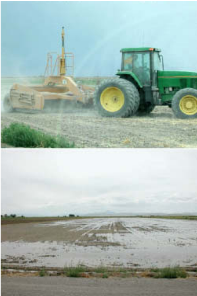
The combination of laser land-leveling and recent advances in surface irrigation provide a hydraulic performance comparable to sprinkle irrigation. (Photos of laser land-leveling equipment [above] and surface irrigation of a leveled field [below] courtesy of Wynn Walker, Utah State University.)
